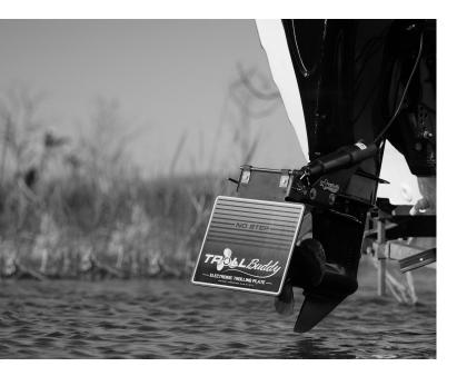
The Trollbuddy system, consisting of a linear actuator, microprocessor control option, and aluminum plate assembly, adjusts trolling speeds on both outboard and inboard/outboard motors to maintain optimal trolling speed.
