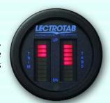
TAB POSITION INDICATOR 2 1/4" diameter. Eight LED's indicate port and starboard tab position. Can be used with, or retrofitted to, any 4 or 8 second Lectrotab installation. Typically used with the basic panel. Display dims automatically at night.
