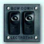
**BASIC PANEL** Two rocker switches in a panel, which is 3 1/8" x 3 1/4" high. Black semi-gloss finish. Switches are also available individually. Switches meet mil-std 202F for salt spray.
