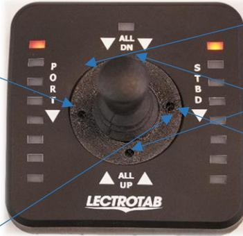
Independent Tab Control: Push and hold joystick 45° towards upper left corner for 4 or more seconds to enter program mode.
