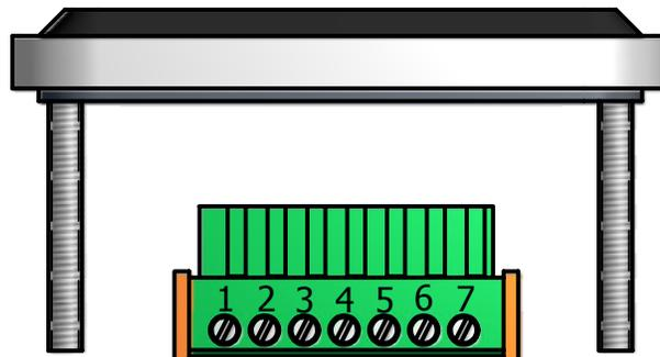
Optional: Connection to ignition key switch to initiate automatic tab retraction. Note: Tabs will automatically retract if the boat is stopped after a few minute delay if this connection is not used.
